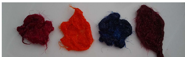
Figure 6. BSA fibers dyed with commercially available acid dyes (left to right: C.I. Acid Red 182, C.I. Acid Orange 7, C.I. Acid Blue 12, and C.I. Acid Violet 12). [Color figure can be viewed in the online issue, which is available at wileyonlinelibrary.com .]
